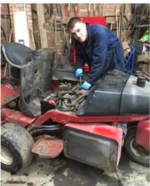
The cutting units will all be removed, ready for a mobile regrinding company to come in shortly.
